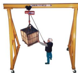
Rigging on gantry crane Source: WA LNI
