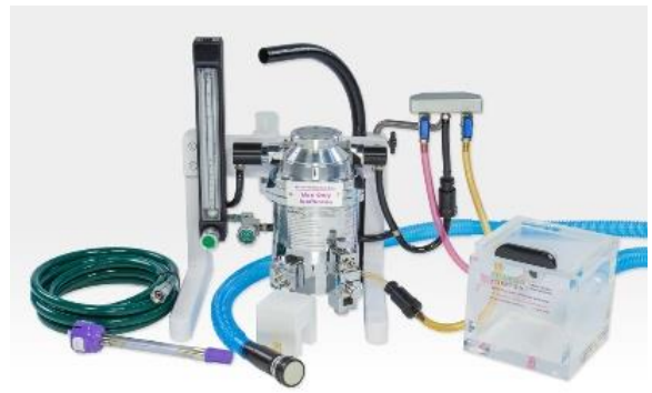
Image 13: Scavenger attached to local mechanical exhaust gas scavenger
