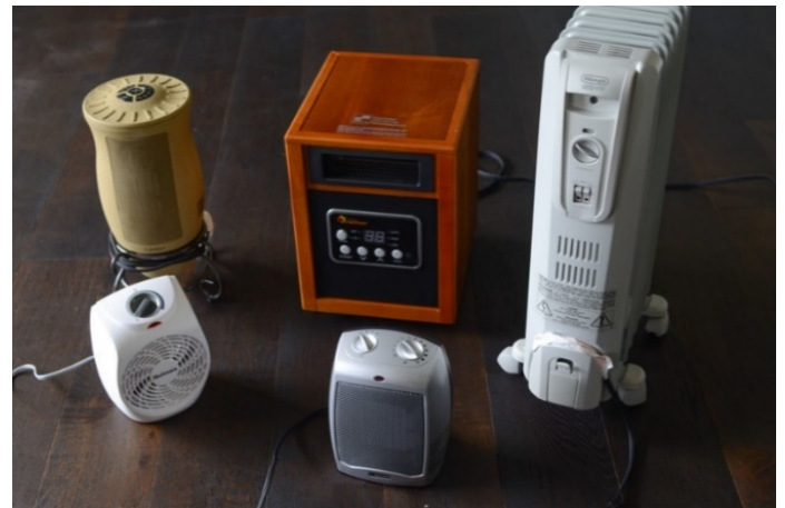
Examples of standard space heaters that require 3 feet of clearance from combustibles
