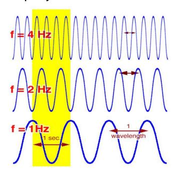
The number of waves that pass a fixed point during an interval of time is referred to as the wave frequency (f or the Greek letter  $\nu$ ). Frequency is measured by counting the number of waves that pass a fixed point in one second. From one wave crest to another is called a cycle, so frequency is often described as cycles per second (or Hertz). One wave, or cycle, per second would therefore have a frequency of 1 Hertz (Hz).
