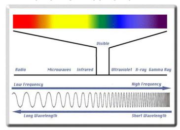
Like ionizing radiation, such as x-rays and gamma rays, NIR is a part of the electromagnetic (EM) spectrum and is propagated as waves through a vacuum or some medium. However, NIR differs from ionizing radiation because it consists of lower quantum energies and, therefore, has different biological effects. NIR displays its own unique personality.
