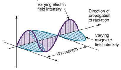
Electromagnetic radiation is the propagation of energy. This energy consists of oscillating electric and magnetic fields, which are transverse and perpendicular to each other. An electromagnetic wave is essentially then made up of fields which are inter-related and interdependent. Both fields can exert a force. An electric field can affect an electric charge (for example, an electron). And a magnetic field can, in turn, affect a moving charge (current).
