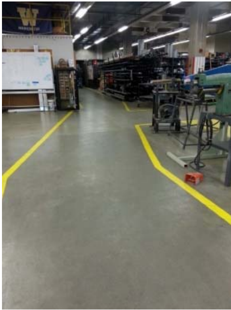
Floor marking indicating safe walkway.
